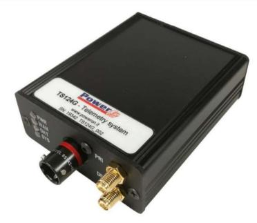
TS124G is a 4G device used to send telemetry data in real time. It allows data transmission to one or more connected PCs and, if covered by 4G Network, the transmission occurs in any place. Regarding data receiving, only an Internet connection is necessary.
