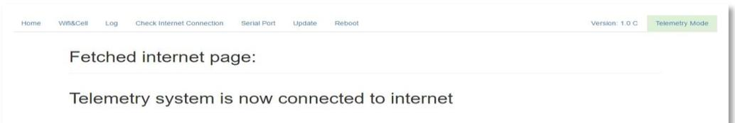
By clicking on “Check Internet Connection”, this screen will be displayed. In this page it is possible to verify if the device, after having set up the correct APN, is connected to the network.
